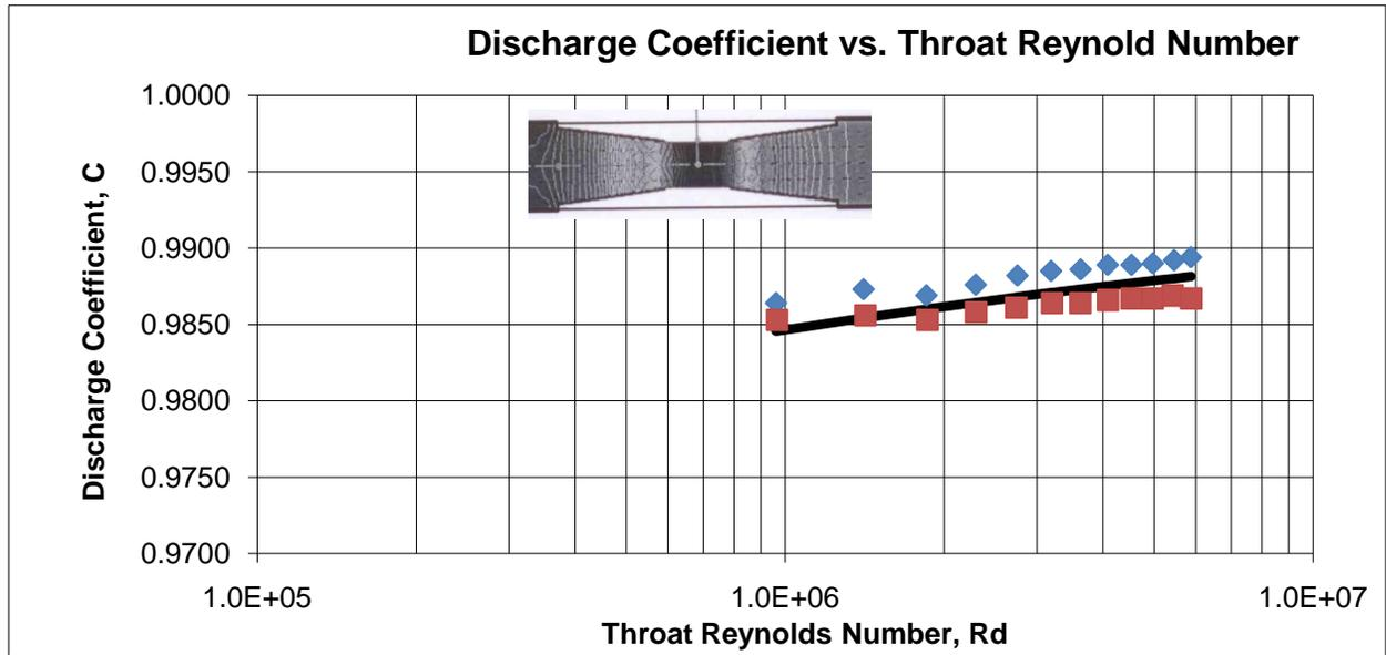
Figure 2 Discharge coefficients for AMITY's Bi Directional flowmeter.
