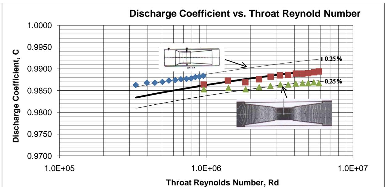
Figure 1 Discharge coefficient for AMITY's Bi Directional flowmeter.
